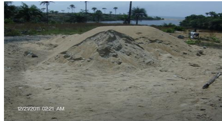
Deposit of beach sand for construction works
