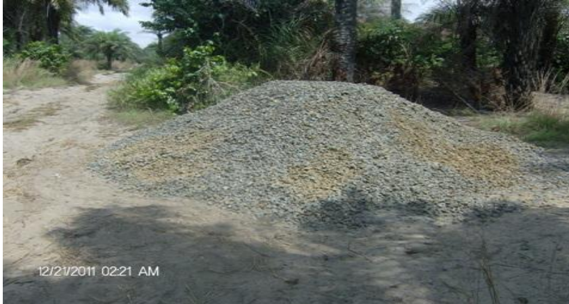
Deposit of crushed granite rocks for construction works.
